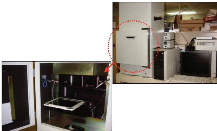
Figure 1. A, Olympus OV100 whole-mouse imaging system. See text for details. B, OV100 covers a wide range of magnifications, from \times 0.14 ( 63 \times 47 mm imaging area) to \times 16 ( 0.6 \times 0.45 mm). Five individually optimized objectives, parcentered and parfocal, provide a 106-fold magnification range for seamless imaging of the entire body down to the subcellular level without disturbing the animal. The optics and antireflective coating ensure optimal imaging of multiplexed fluorescent reporters in small animal models. Subcellular structure can be visualized clearly by fluorescence imaging.
